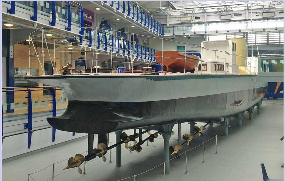
Turbinia , on display at the Newcastle Discovery Museum, showing her unique triple-shaft, triple-propeller arrangement.
